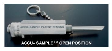
ASTM Aviation Fuel Particulate Contamination test method D 2276, A2.3 requires a sample point. Part 2.3.1 states ... "Care should be taken in such cases to avoid trapping or general contamination"... and 2.3.2. "Sample Valve Connection...must have a minimum of internal recesses which could cause the hold up of contamination"....
